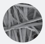
**Microscopic view** Thermal bonded filaments for excellent pleat stability
