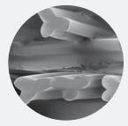
**Cross section** Filtura filter medium with trilobal filaments for enhanced filtration efficiency and dirt holding capacity Pool & Spa filter media portfolio
